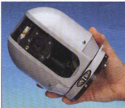
Controp's D-STAMP payload is optimised for installation on board small-sized UAVs and equips the Aeronautics Orbiter, Rafael Skylite and Elbit Skylark aircraft.
